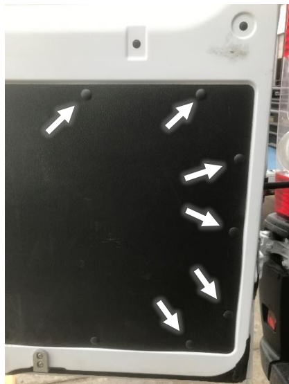
Figure 19: Remove Plastic Door Rivets
