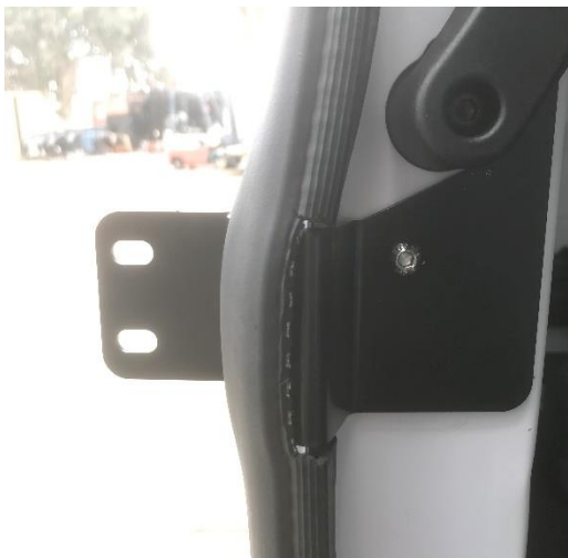
Figure 15: Installed Weather Stripping After Modification
