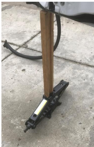
Figure 2: Support Door Prior to Installation
