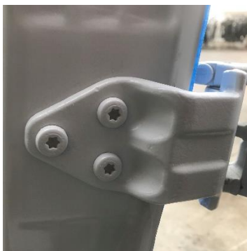
Figure 8: Inside View of Lower Hinge
