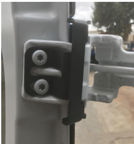
Figure 7: Inside View of Installed Upper Hinge Bracket
