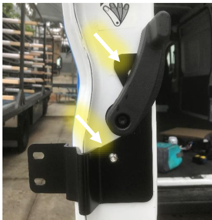
Figure 12: Inner Driver Door Bracket Installed
