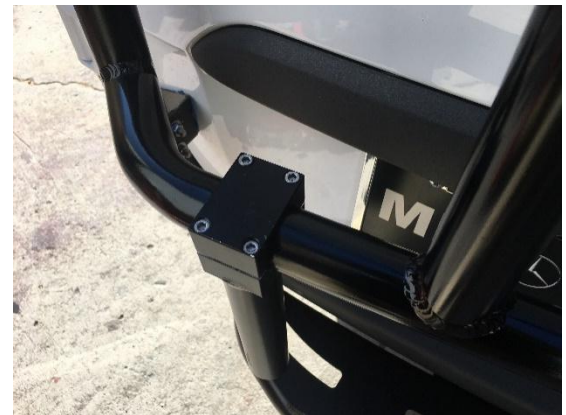
Figure 1: Bolt-On Supports Loosely Bolted to Lower Crossmember
