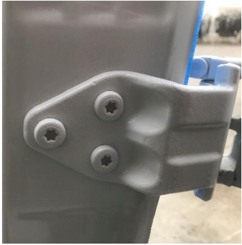
Figure 8: Inside View of Lower Hinge
