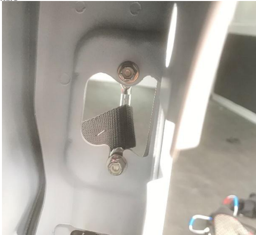
Figure 21: Backside View of Door Stop Mounting
