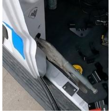
Figure 11: Clamp Lever Mounting Post
