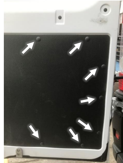
Figure 19: Remove Plastic Door Fasteners
