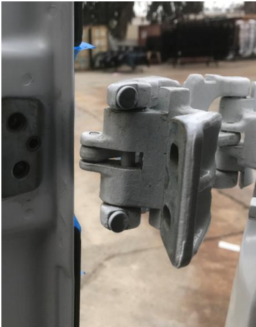
Figure 4: Upper Hinge Rotated Away from Door
