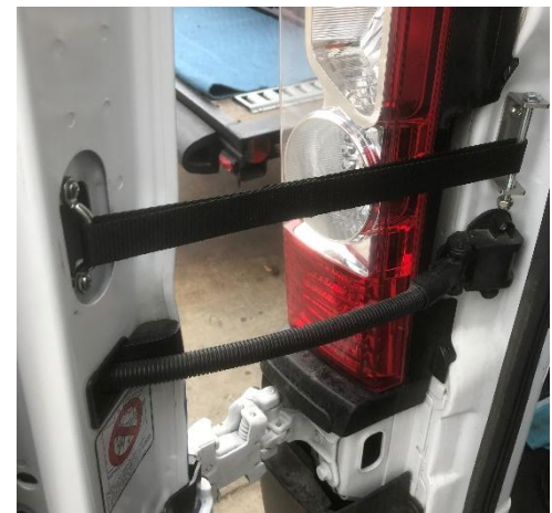
Figure 24: Complete Door Stop Install
