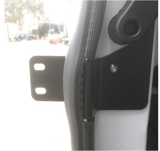
Figure 15: Installed Weather Stripping After Modification
