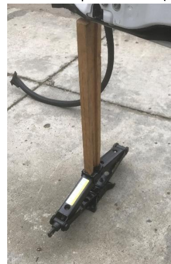
Figure 2: Support Door Prior to Installation
