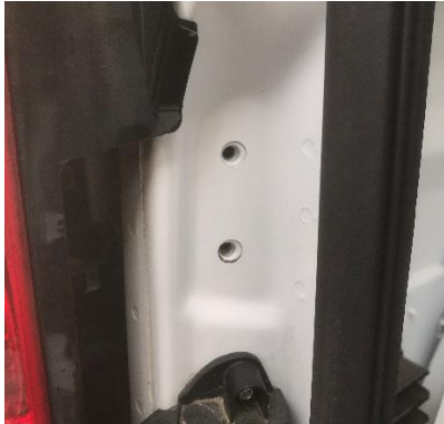
Figure 17: Factory Threaded Holes
