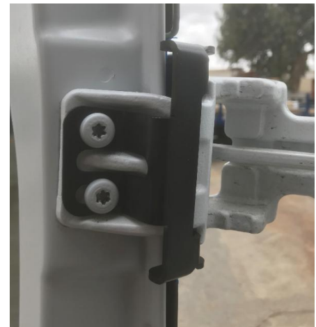
Figure 7: Inside View of Installed Upper Hinge Bracket
