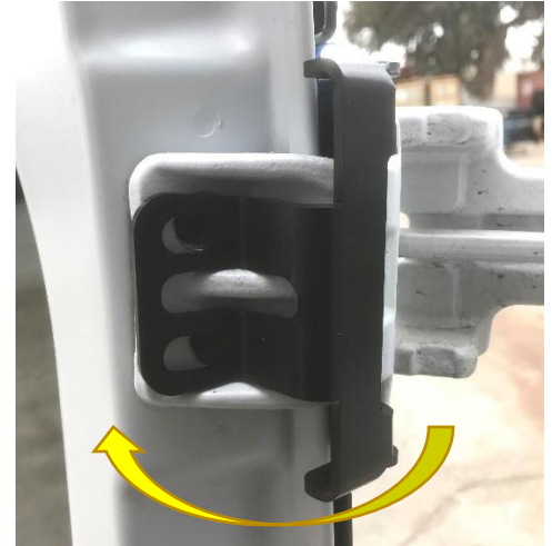
Figure 6: Bracket Installed Over Factory Hinge
