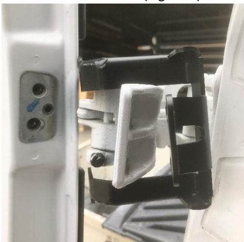
Figure 5: Bracket Installed Over Factory Hinge
