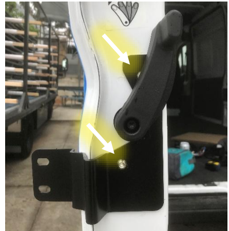
Figure 12: Inner Driver Door Bracket Installed
