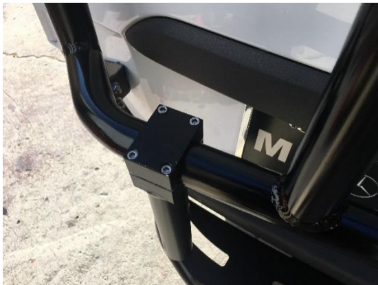
Figure 1: Bolt-On Supports Loosely Bolted to Lower Crossmember
