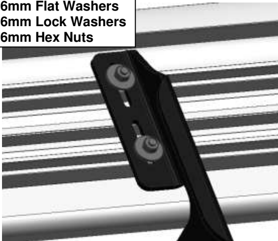
(Fig 13) Attach Running Board to Brackets
